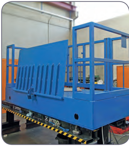
vehicle loading lift
